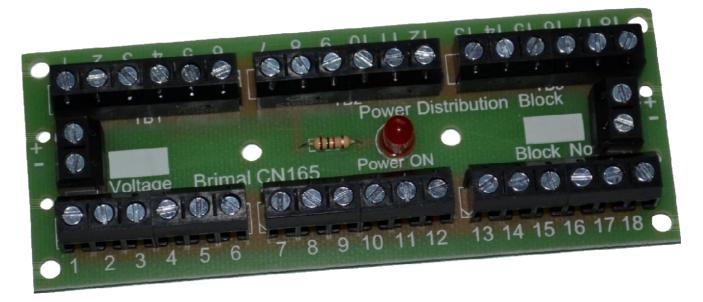
Fixing holes are 3.5mm diameter so will accept M3 screws.
