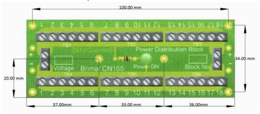
The two holes at each end are for cable ties to Secure the input cable
