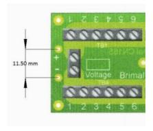
Brimal Consultants Ltd trading as BRIMAL COMPONENTS. 60 Lawson Road, Seaton Carew, Cleveland, TS25 1AL Telephone: 01429 297 277. Email Andrew@brimal.co.uk This drawing shows how the CN165 can be used as a distribution point in a Bus Bar system. The Bus Bar comes in on the left and goes out on the right, with 18 spur off points now available, to feed all the equipment in that area of your Layout.
