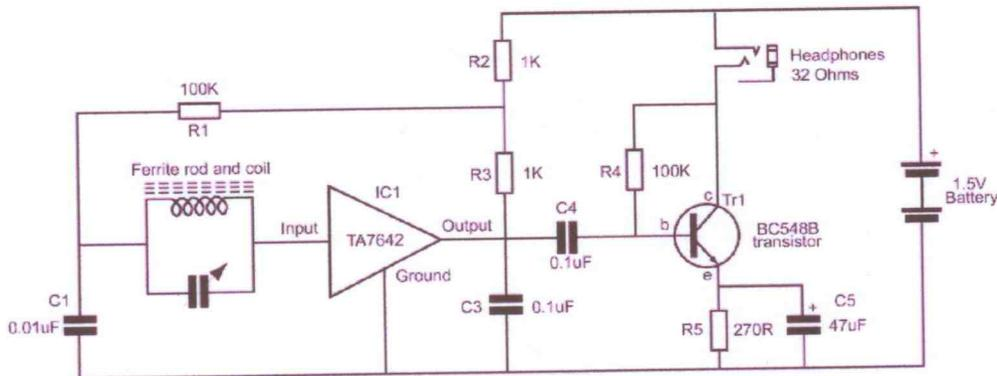
The coil needs approximately 55 turns of 0.315 (30 SWG) of enamelled copper wire on a 100 x 10mm ferrite rod. A process of trial and error will help you achieve the optimum number of windings.
