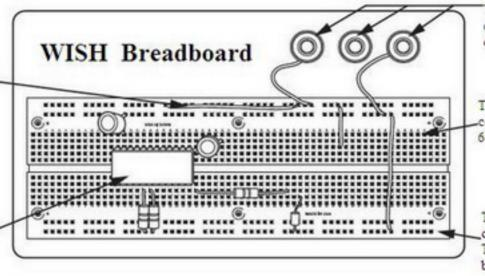
Three binding posts for connections to power supplies or external equipment.
